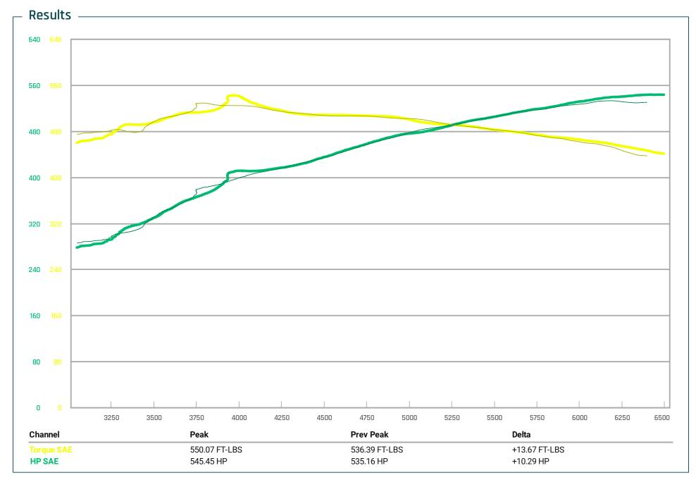
Note: MPI lid had an increase in about .25-.5 lbs of boost. Custom lid generates better flow and caused more knock detection on the stock tune which resulted in about 1 degree of timing retard and power back. This shows the lid is superior to a OEM lid. 2015-2016 LT4 engines in the ZO6 had a shorter lid. MPI lid has proven to be a huge upgrade for older, shorter lid design engines.
